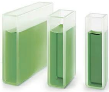
Figure 16: Visual image of 10mm, 20mm and 50mm cuvette cell (Merck, 2024b)
