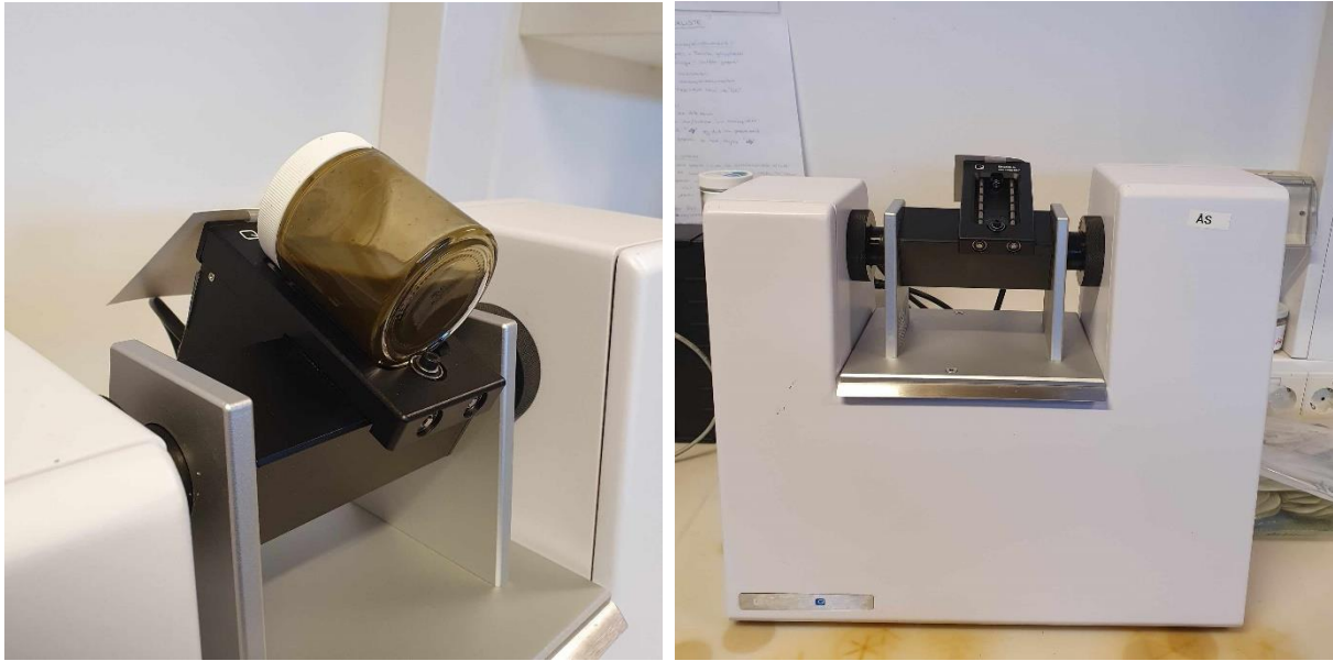
Figure 3. NIR measurement with Q-Interline's Quant FT-NIR Analyzer equipped with the bottle sampler.
