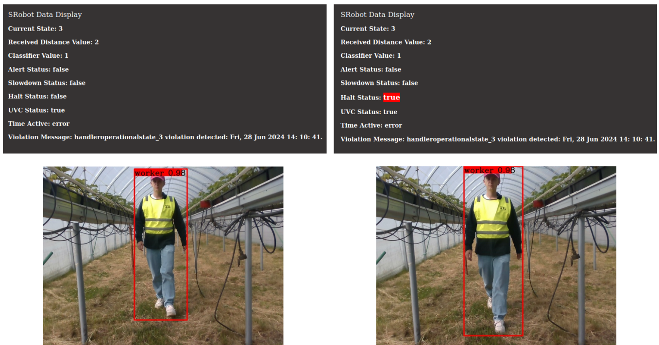
Fig. 51: Compiled screenshots of front-end showcasing the first violation scenario triggering a handler, correcting the safety controller to publish to the halt topic.
