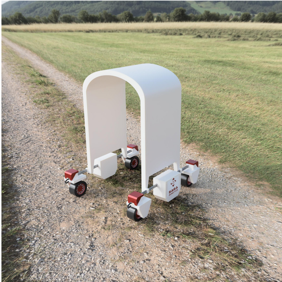
Fig. 31: Fusion 360 model of the Thorvald robot, used for demonstration in the gazebo environment.
