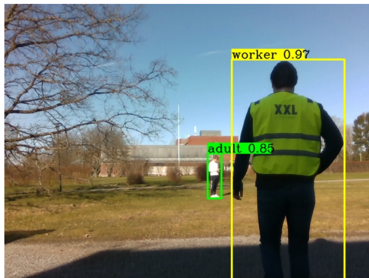
Fig. 53: Classification of a worker and an adult, differentiated by a safety vest, at noon.
