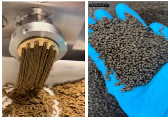
Figure 5: Pelleting of mixed ingredients without cutting (left); pelleted feed after drying (right).
