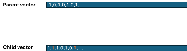
Figure 1: Illustration of mutation of genes (features included or not). The blue lines signify chromosomes (solutions), while the change in genes is highlighted in orange.
