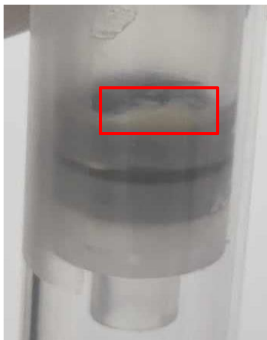
Figure 21. Shows yellow-white starch (red box) stuck in the spin column filter after centrifugation.
