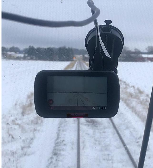
*Figure 3: Nextbase 522GW dashboard camera mounted on the front shield of a train at Kinnekullebanan railway (foto by Elise Lyng Monssen).*
