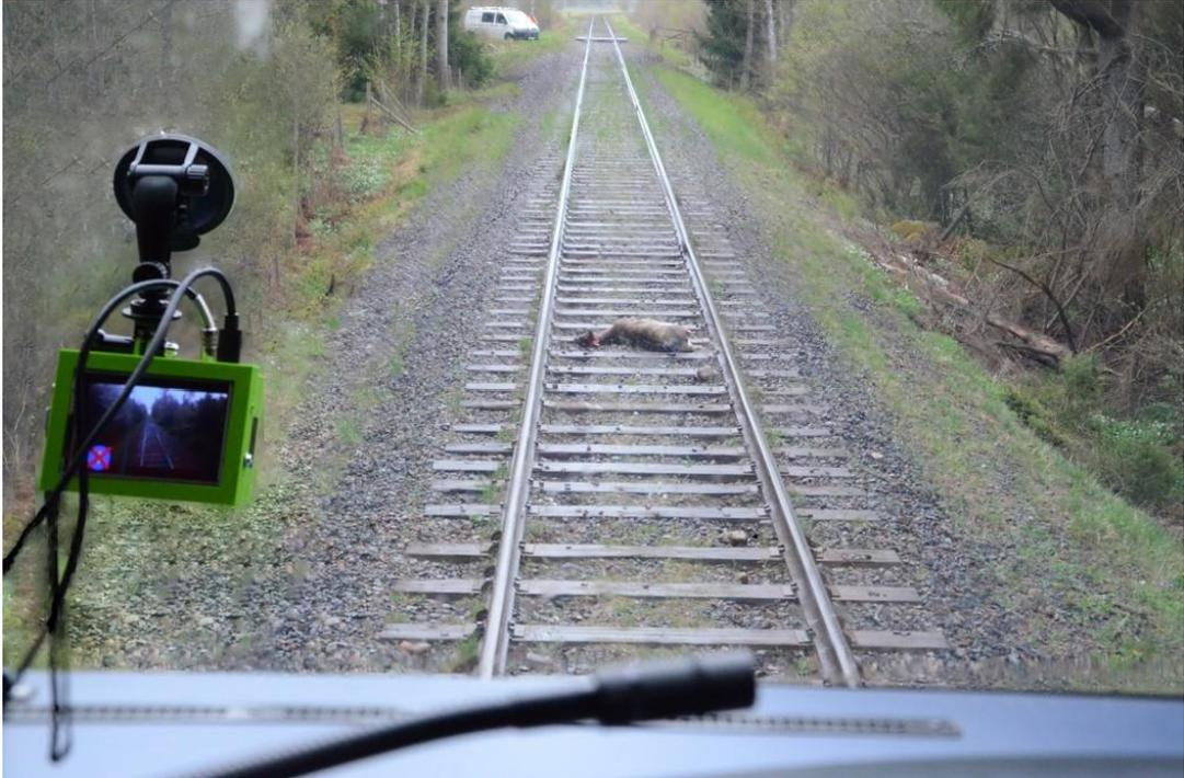
Figure 2: DASS-unit mounted on the front shield of a train, filming a dead fallow deer on the railway track (foto by Mathias Olsson).
