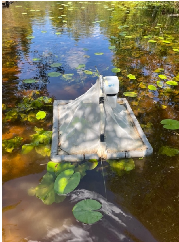
Figure 3. An emergence trap floating on the surface of a sampling site included in this study, photo: Kåre-Jørgen Ingerø Bøe.
