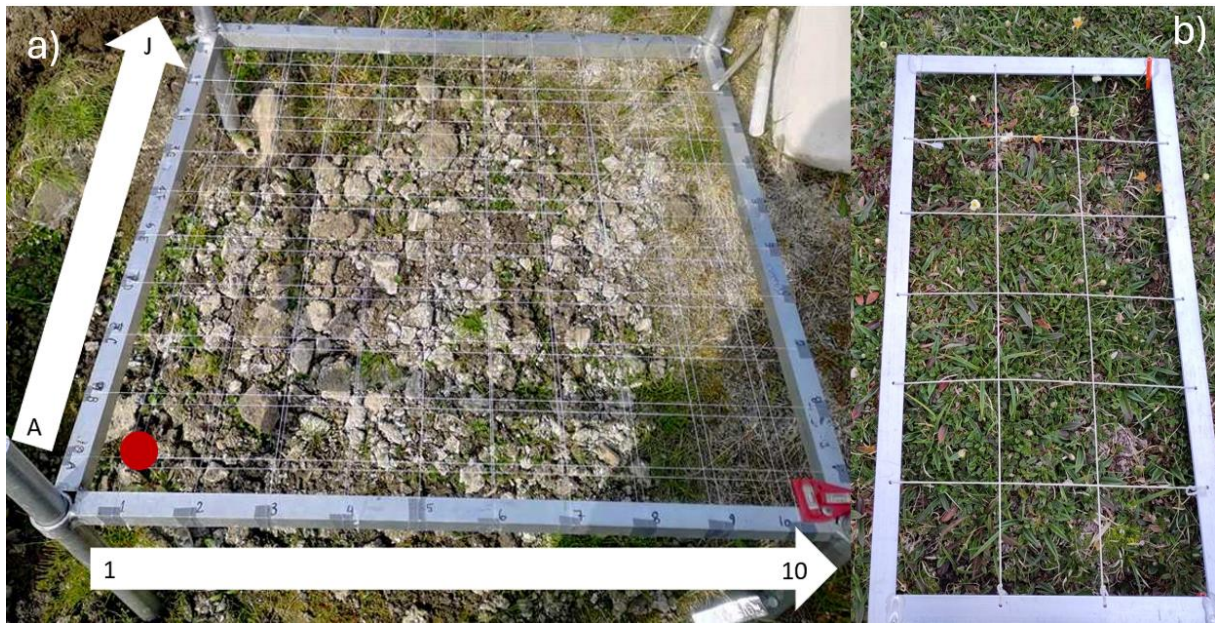
Figure 4: a) The point intercept frame used when conducting vegetation analysis in the High Arctic site. The red spot represents where the recording started. The frame was divided into 10×10 squares, from A1 to J10. Photo: Merle Scheiner. b) The frame used for vegetation analysis in the alpine site. The frame was 30×60 cm and used for recording one sub-plot at a time. Photo: Gaute Eiterjord.
