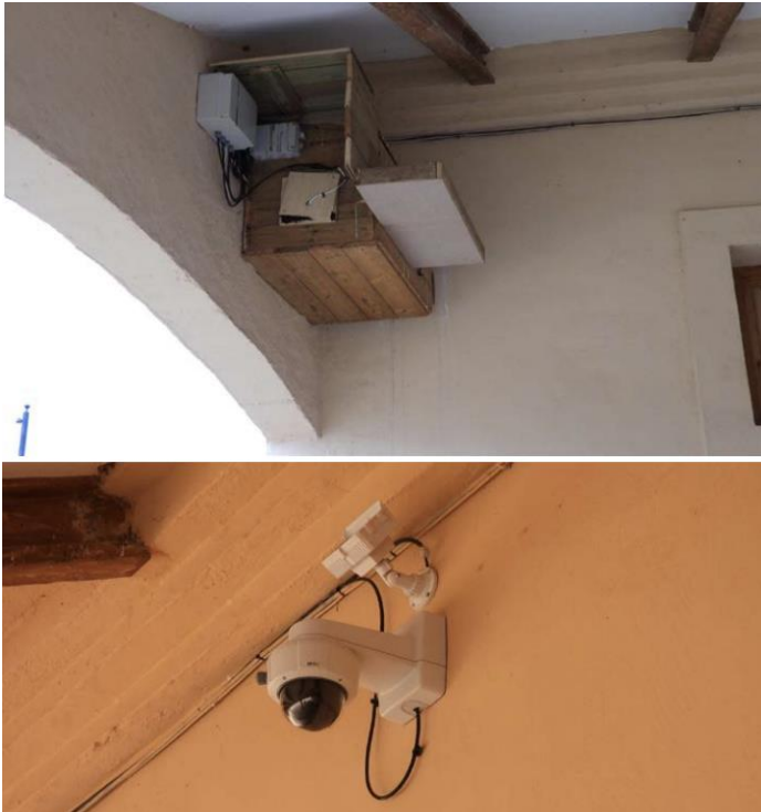
Figure 2: Photo of the nest box and camera setup at the Cabaneros nest in 2023. The upper photo shows the nest box with the installation of the interior camera. The lower photo shows the exterior camera. Photo: SEO/BirdLife.
