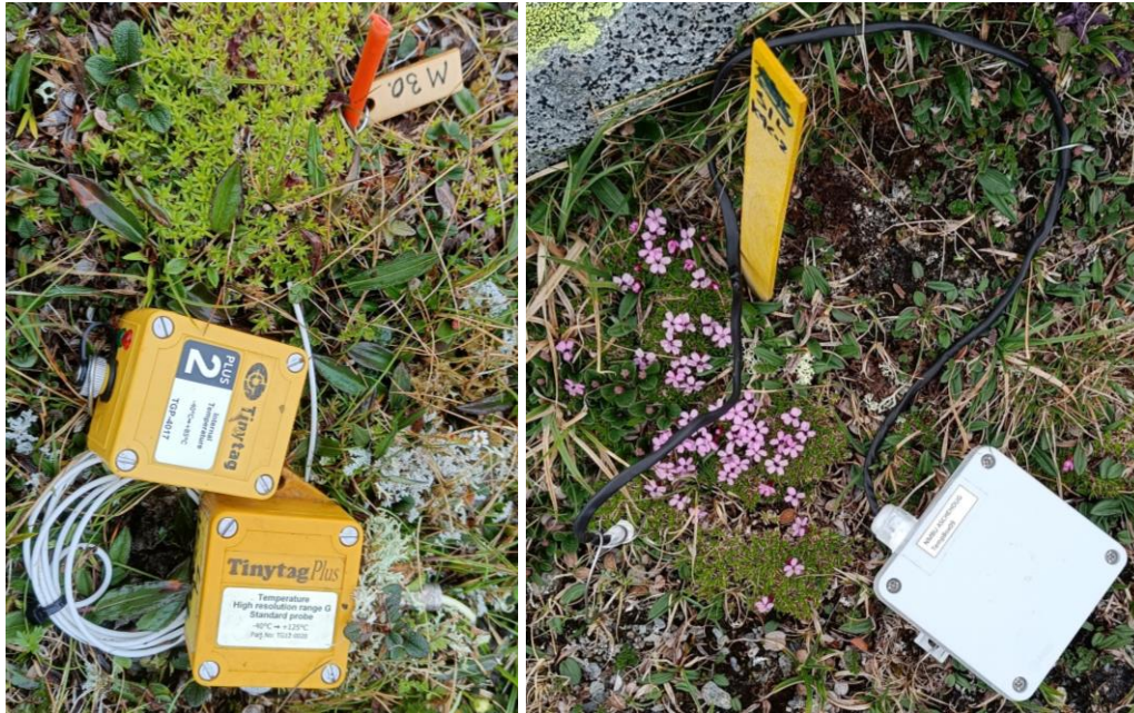
Figure 7: Ambient- and in-cushion Tinytags (left) and DIY TempBox (right) in placed by S. acaulis plants in the field.
