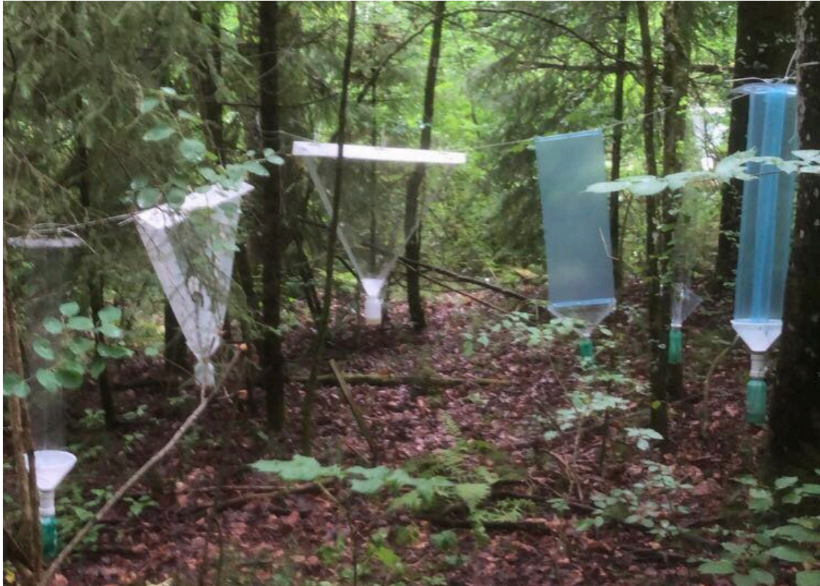
Figure 3. The set-up of all six trap types at one sampling location. From left: Cross-PC, triangular-PE, triangular-PC, rectangular-PE, rectangular-PC, and cross-PE.
