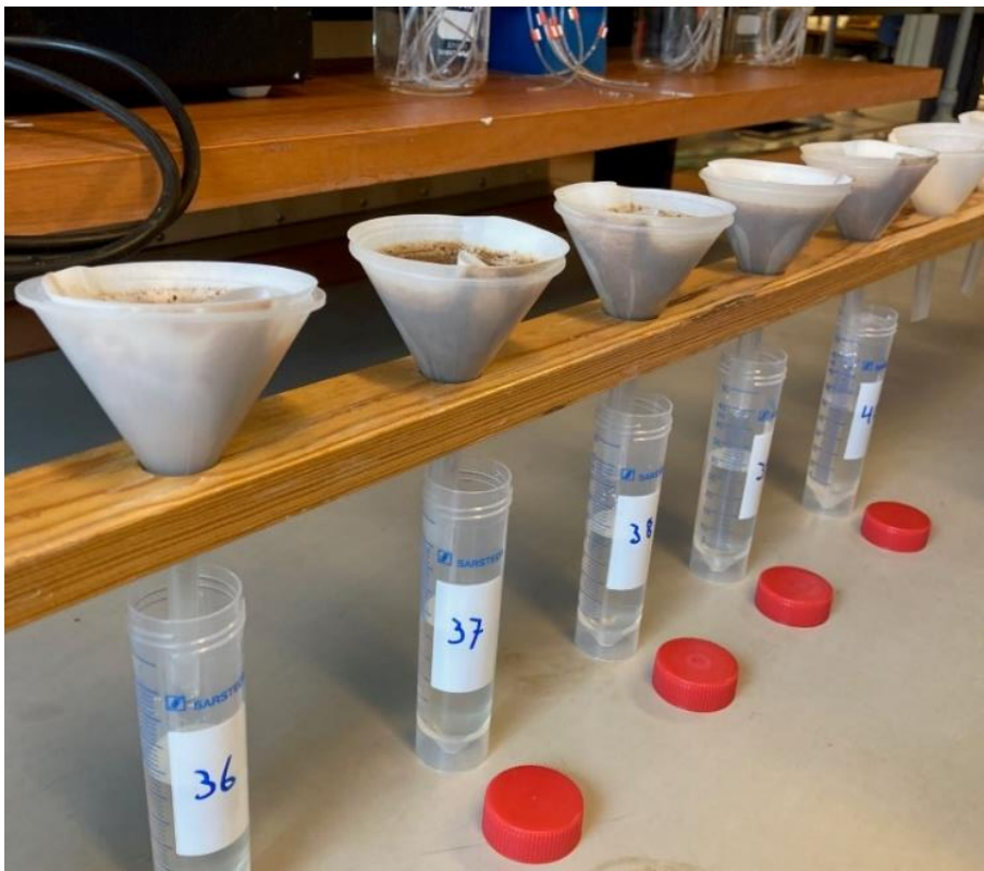
Figure 11: Paper filters in plastic funnels over plastic beakers to filter out soil particles.
