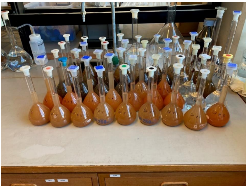
Figure 10: The samples in measuring bottles (250 ml) ready for spectrophotometry. The orange solutions in front are burned samples for inorganic P and the darker solutions in the back are unburned for total P.
