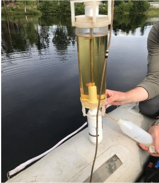
Picture 1 - Showing a full water fetcher, where 0,5 L was transferred into pre-washed plastic bottles.
