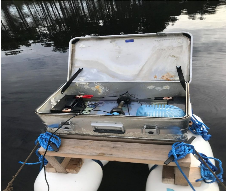
Picture 2 - Automatic vertical profiler with a YSI 6920 multiprobe
