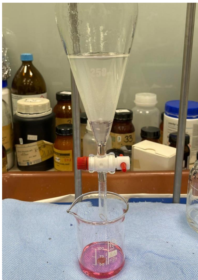
Figure 8: Separation of the pink I 2 organic phase to the beaker. The remaining organic phase in the funnel (bottom) became transparent, indicating complete separation of I 2 to the beaker. Photo: J. Lauritsen.
