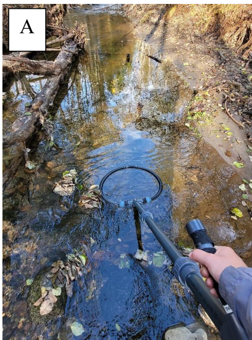
Figure 4. A: Manual PIT-scanning was conducted using an Oregon RFID HDX Single Antenna PIT Tag Reader kit. B: The receiver was kept in a backpack with a rechargeable battery. Photos: Ole Eivind Ovnan Fjeldstad.
