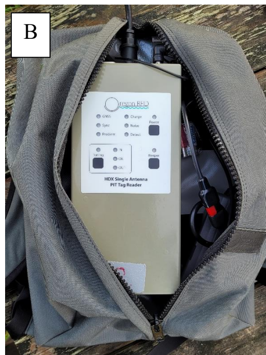
Figure 4. A: Manual PIT-scanning was conducted using an Oregon RFID HDX Single Antenna PIT Tag Reader kit. B: The receiver was kept in a backpack with a rechargeable battery. Photos: Ole Eivind Ovnan Fjeldstad.
