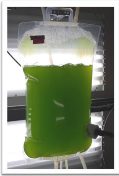
Images 1: Top left: Tubular (vertical) photobioreactor (); Top right: Flat panel photobioreactor (Ruhr universitat Bochum); Bottom: Plastic bag photobioreactor (Cellana)
