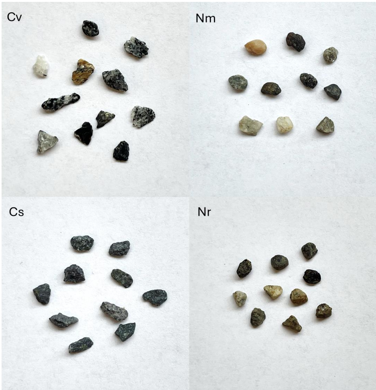
Figure 18: 2D picture of sand particles >2 mm to demonstrate the differences in particle shape between two types of crushed sands (Cv and Cs) and two types of natural sands (Nm and Nr). Foto taken by Sigrid Esmeralda Arnestad.
