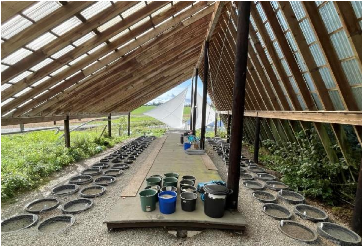
Figure 3: Experiment site at NMBU with 2x48 lysimeters on each side of a cellar that functioned as a control room for water drainage. Picture taken from the back (northeast). Photo: Sigrid E. Arnestad.
