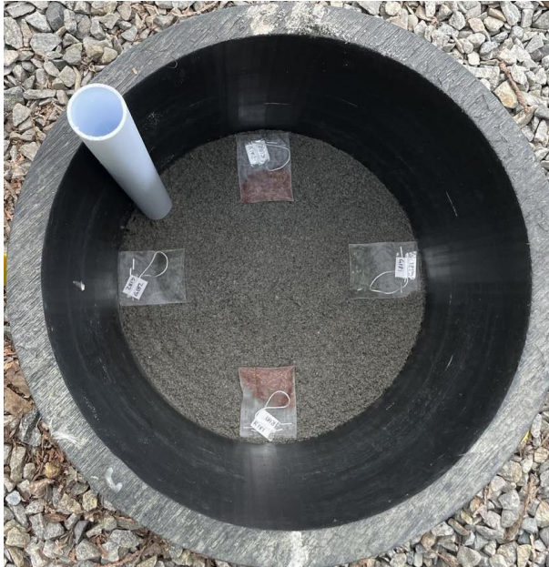
Figure 6: Demonstration of the placement of the teabags (left), with two replicates of both green tea and rooibos buried against the wall with the labelling facing upward. The illustration of the lysimeter (right) show visually the design of the teabag experiment, with the two tea layers (T1 and T2) and corresponding volumes of soil. The water level (blue line) was controlled to be 15 cm from the lowest part of the bottom of the lysimeter.
