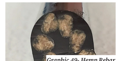
Graphic 49- Hemp Rebar Including hemp has proven to reduce corrosion, tripling a structures lifespan (Aouf, 2022)
