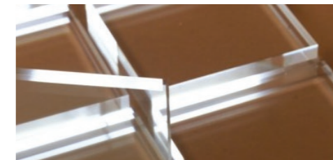
Graphic 101 - Transparent Aluminium Its fully see-through, 3x harder than steel, used for armored windows and optical lenses (Neenu S K, 2022)
