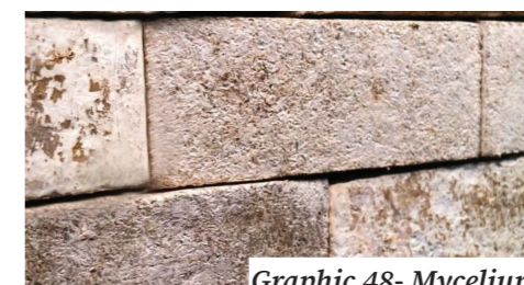
Graphic 48- Mycelium Mushroom roots can be cultivated on any local organic waste and be shaped to any form for insulation, furniture.
