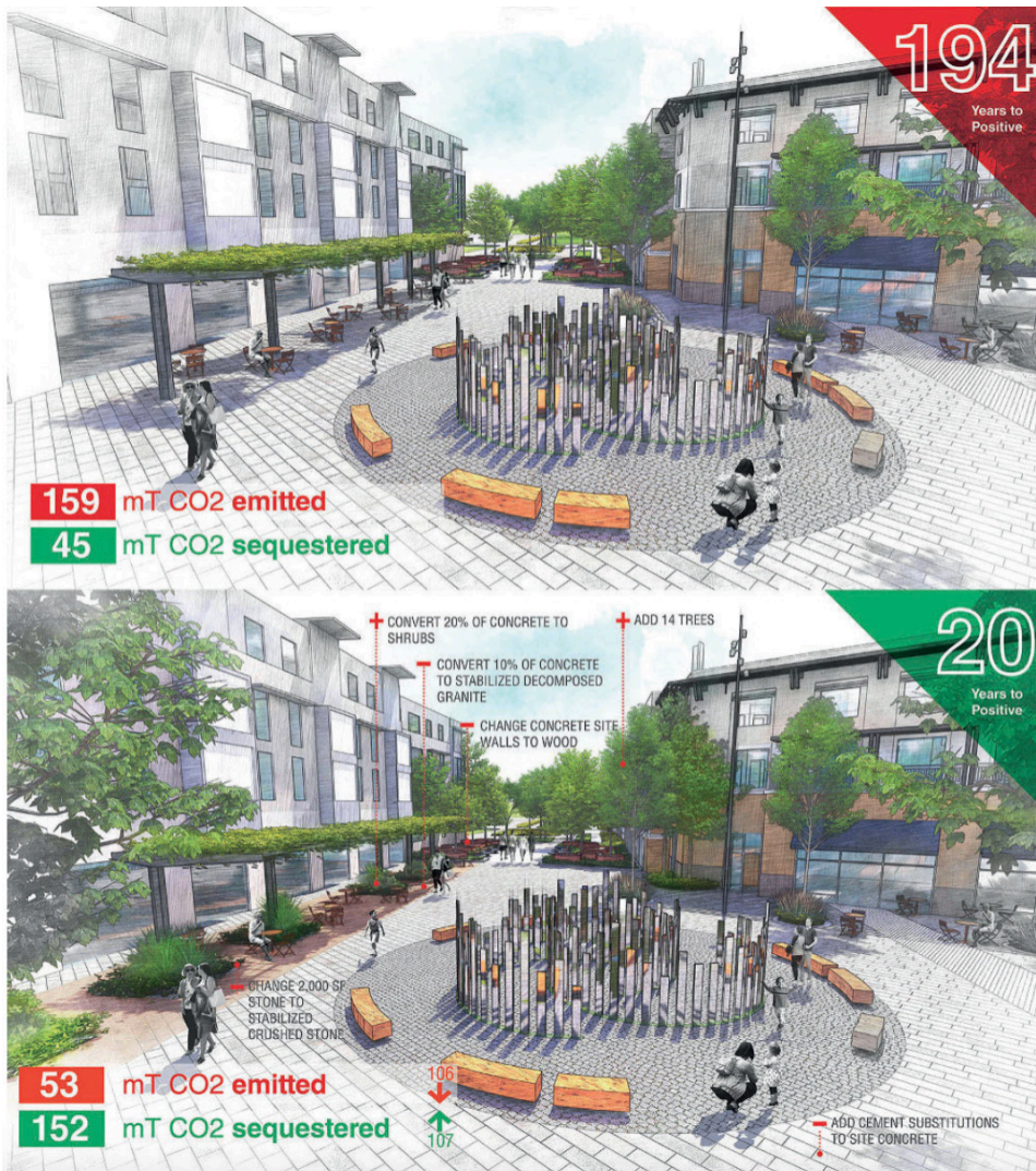
Figure 15. Two different design scenarios and the corresponding number of years until carbon positive. Source: Norconsult Norge AS, Klimapositive byrom i Horten kommune. (Used with permission)
