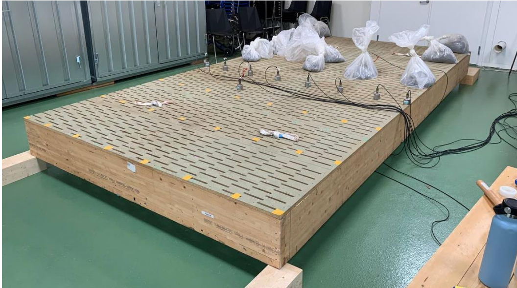
Figure 3-15. Model04 on floor G106 using sandbags.
