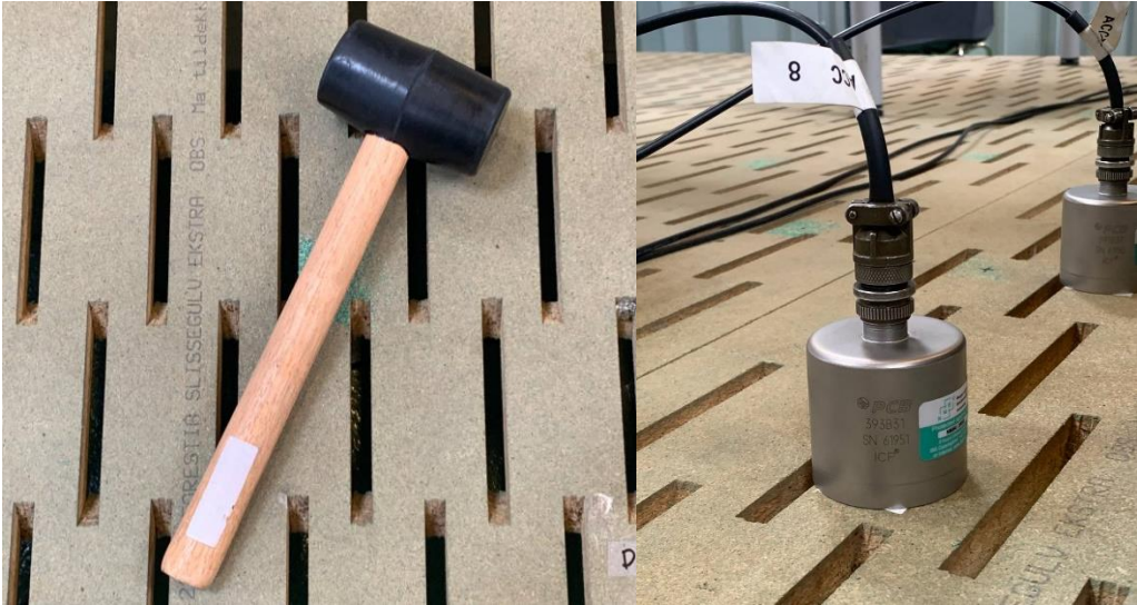
Figure 3-7. Rubber hammer and accelerometers used for testing.
