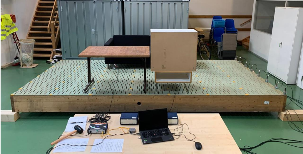
Figure 3-8. Floor G101 during hammer test.
