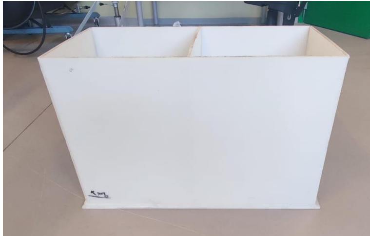
Figure 4. 21: Side view of the fabricated MBBR and sump
