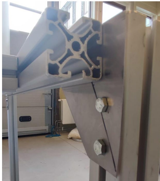
Figure 4. 17: Bolt and nut to join separate aluminum frames I.
