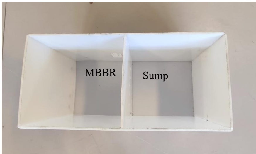
Figure 4. 22: Top view of the fabricated MBBR and sump
