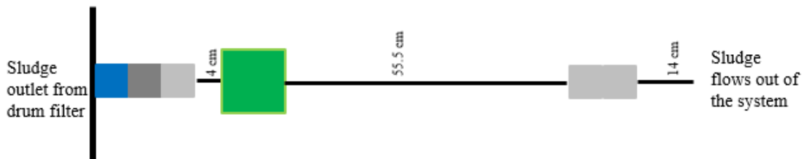
Figure 4. 33: Drum filter to sludge outlet pipe layout.
