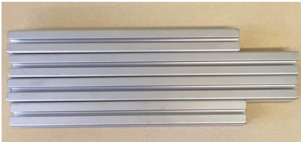
Figure 4. 13: Aluminium pipes used for the RAS support framework.
