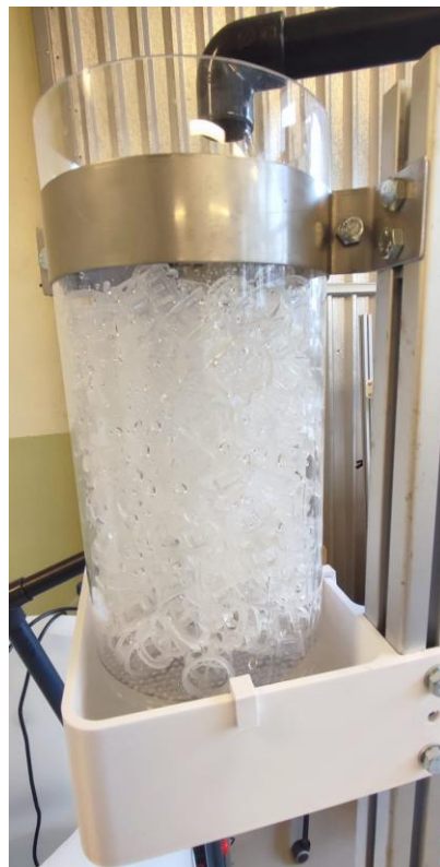
Figure 4. 28: The degasser with media and the 3D water retainer attached to the aluminium pipe frame.
