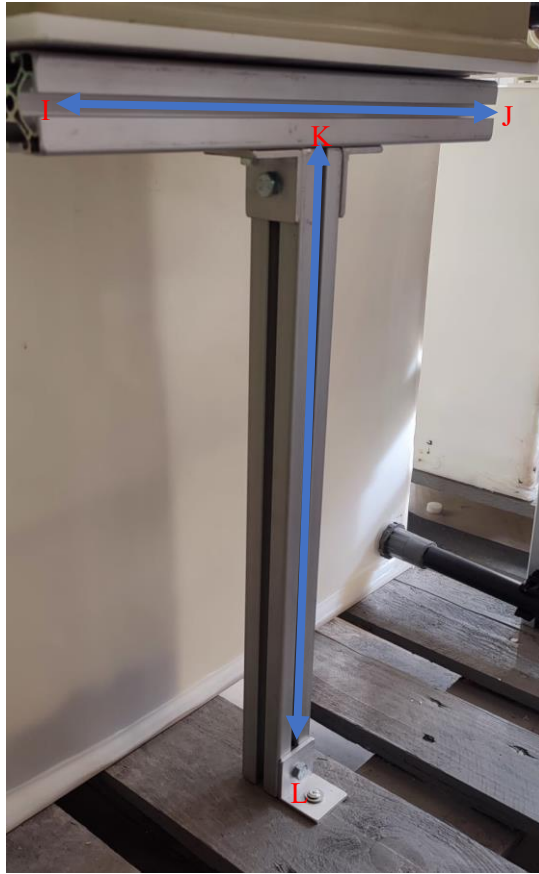
Figure 4. 23: T- support frame for mechanical filter
