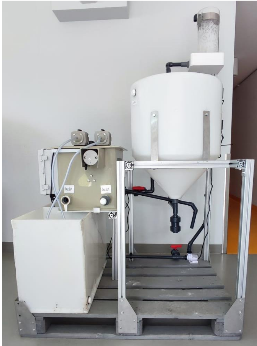
Figure 5. 2: The left-side view of the finished RAS unit.
