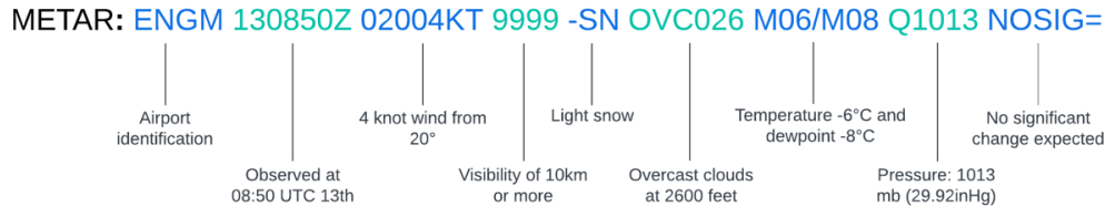
Figure 2: An example of a METAR message and how to decode it.
