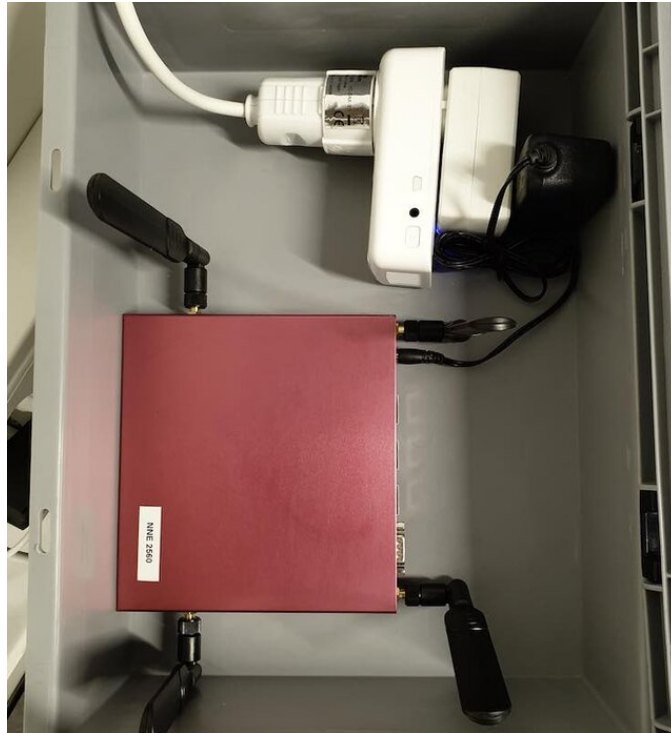
Figure 4.1: A measurement box with an NNE node and a power source (Ahmed and Pathan, 2019)
