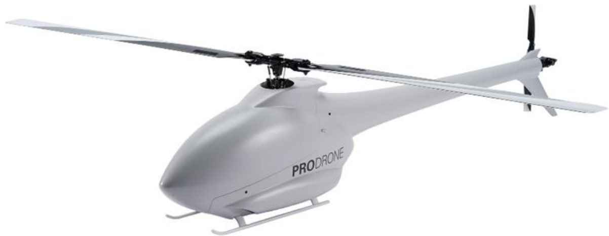
FIGURE 4: AN EXAMPLE OF SINGLE ROTOR DRONE, THE PRODRONE PDH-03 [10]
