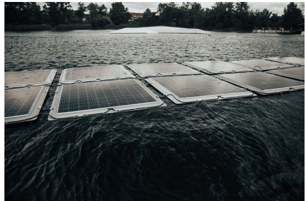
Figure 10: Horizontal panels on aluminium floats from Sunlit Sea. With permission from [9].
