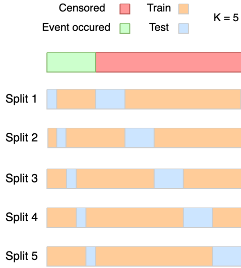
Figure 2.7: This figure demonstrates the Stratified K -fold cross-validation process using k = 5 folds. Each split represents how the dataset is divided into training (orange) and testing (blue) segments. This method ensures that the proportion of each class (censored and event occurred) is consistent across all train and test sets, reflecting the overall distribution in the complete dataset.
