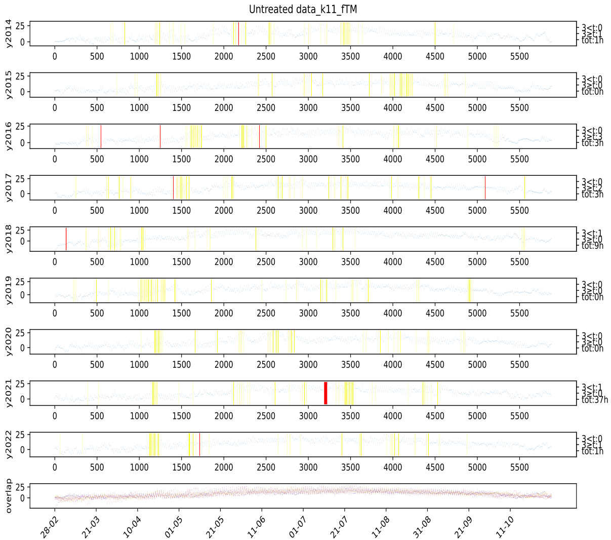
Figure 127: Visual representation of missing values at station 11 from 2014 to 2022 at the parameter "TM" after treating for outliers. The left numbers indicated how many hours that are missing and how many of them are shorter than or longer than 5 hours, however for this visualization they indicate the untreated version of the data. The yellow markings indicate possible outliers based on the given year, all markings was checked if they were actual outliers. The red colouring indicate missing values in the data (represented in the data with code "NULL"). The station names can be found in table 1.
