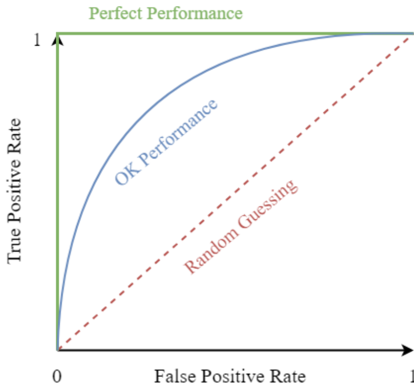
Figure 2.8: Illustration of ROC curves, with the green curve representing perfect performance, the blue curve showing OK performance, while the red dashed line depicting random guessing. Inspired by Raschka and Mirjalili [21].
