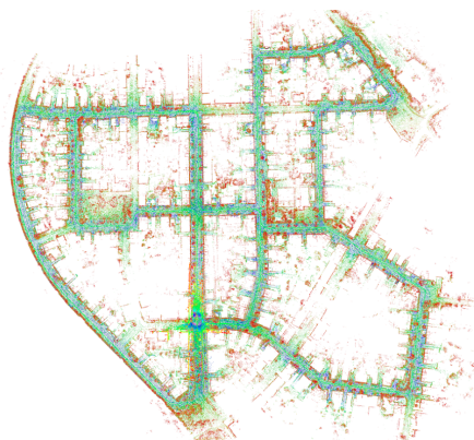
Fig. 10: Resulting map after running A-LOAM on KITTI sequence 00. Image from their GitHub [36].
