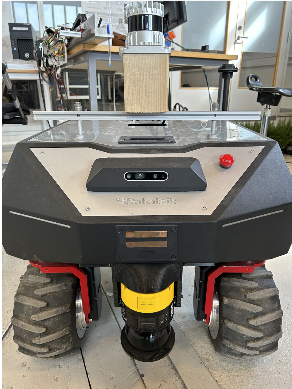
Fig. 21: RB-Vogui with attached Ouster OS0-128 on top and RealSense D435i integrated in the front.
