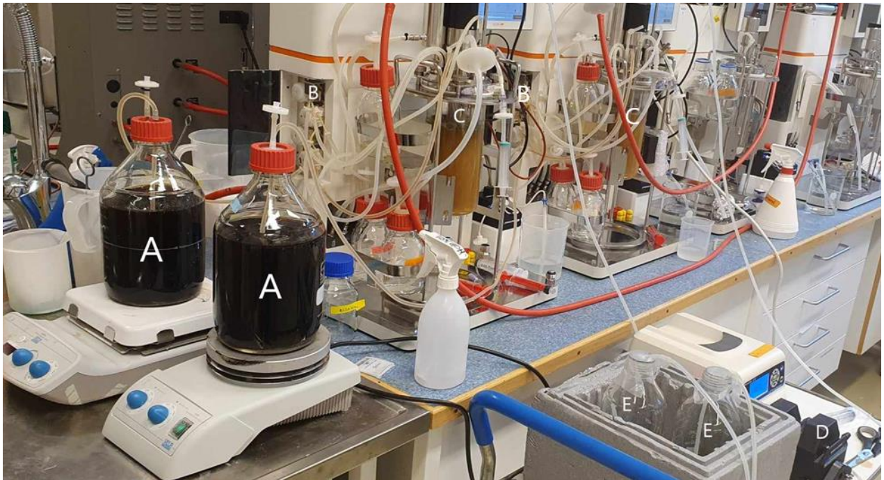
Figure 1. Set-up for the continuous fermentation, with feed bottles (A), peristaltic pumps with tubing leading into the bioreactor (B), bioreactors (C), peristaltic pumps with tubing leading from the bioreactors (D) and waste bottles (E).
