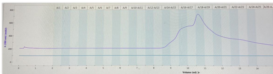
Figure 4.3: SEC chromatogram of cGAS-SUMO fusion protein. The volume (mL) of PBS used during protein elution is represented on the X-axis, while the absorbance measured at 280 nm in milli-absorbance units is presented on the Y-axis. The protein was eluted in fractions of 500 \mu L, and the fractions that showed a peak in absorbance at 280 nm were analyzed using SDS-PAGE.
