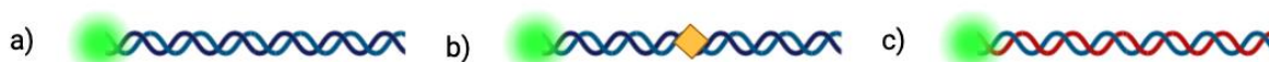
Figure 3.4: Illustration of different 44-mer oligonucleotides with a fluorescent tag. a) complementary DNA, B) complementary DNA with a mismatch at one base pair, and c) RNA-DNA hybrid, where the red strand represents RNA. The fluorescent dye ATTO488 was used to label the DNA strands, while Fluorescein (FAM) was used to color the RNA-DNA hybrid. Both of these dyes emit a green fluorescence upon being excited by light within the blue-to-green range. Figure made in Biorender.com.
