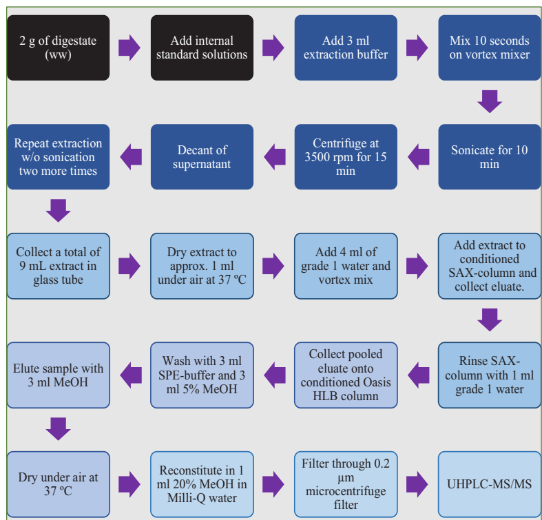
Fig. 1 Flow chart for the extraction of antibiotics and corticoid steroids from biogas digestate, before quantitative analysis with UHPLC-MS/MS
