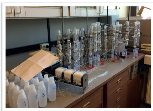
Figure 8. Set-up of the column leaching experiment
