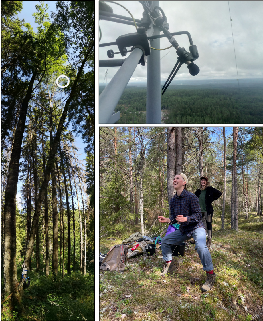
Figure 3. Images depicting different techniques used in this thesis for deploying ultrasonic microphones attached to bat acoustic detectors at heights: on a meteorological tower (top right; Paper I ; Image: Tommy Rambøl) and in the forest canopy ( Paper II ; left, bottom right: using a throw line attached to a 500 g weight for deploying the first in a series of two ropes required for the set up; photo: Katrine Eldegard). The final location of the microphone in the forest canopy detector on the left is indicated with a white circle.
