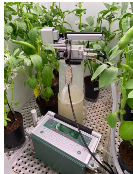
Figure 7: The gas analyzer when measuring light response in the chamber with a low R/BL treatment and ambient \text{CO}_2 .
