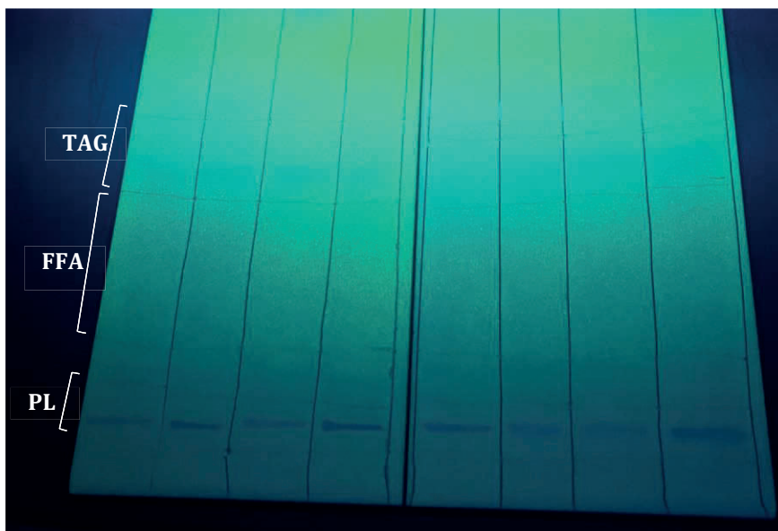
Figure 11. Silica plate sprayed with a fluorescent solution showed, under the UV light, the three separated fractions present in the tested samples (TAG, triglycerides, FFA, free fatty acid, PL, phospholipids).
