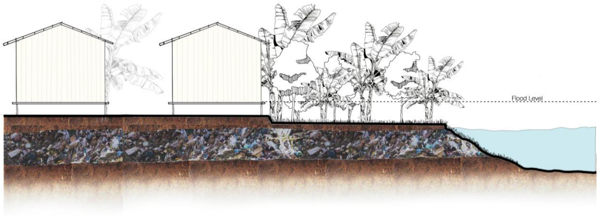
Fig. 80: Flood level where there is enough vegetation between the lake and houses (Zoom 3)
