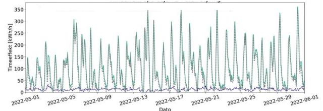
*Figure 3 Power demand for charging (green line), and power demand for heating and service during month of May 2022.*
