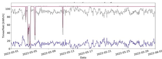
Figure 5 Power demand for the month May showing a few periods where there is available power below the average (purple line). The power for heating and service (blue line) and power for charging (green line).
