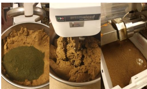
Figure 7: Production of grass protein feed. From powder form to dough and finally to pellets.
