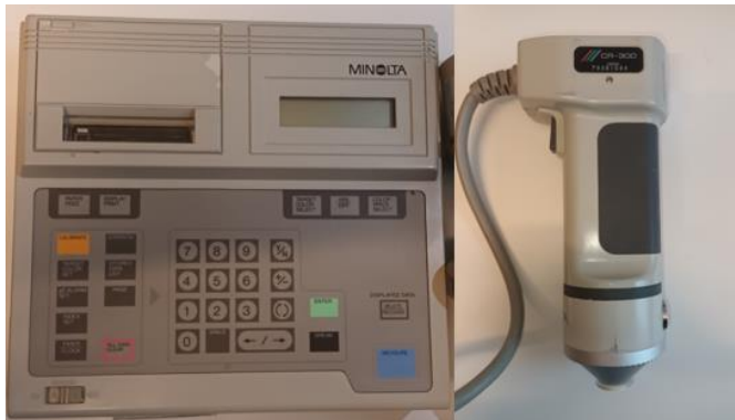
Figure 8: Minolta CR-300 chromameter console and measuring device utilized in the experiment.
