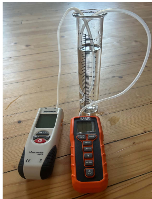
Figure 1. The figure illustrates the setup of our simple yet powerful experiment. We measure the pressure in a fluid cylinder filled with 15 cm of water using three different manometers. Based on new and deeper insights into gravity, we can extract the Planck length without any knowledge of the gravitational constant.
