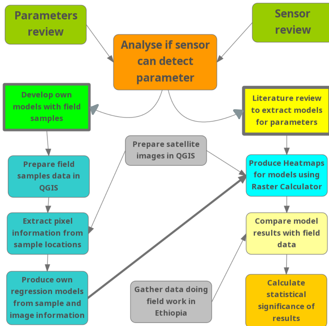
Figure 10 Flowchart of Methodology. Made using mindmup.com
