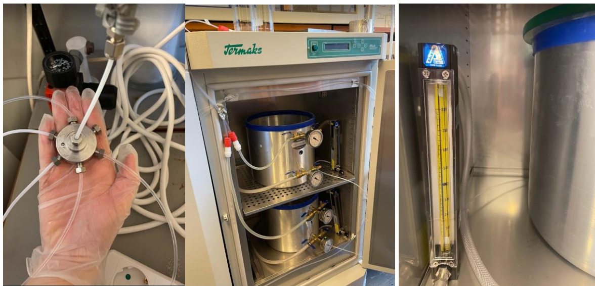
a) Stainless steel splitting brass b) Set up of the vacuum chambers c) Rotameter
