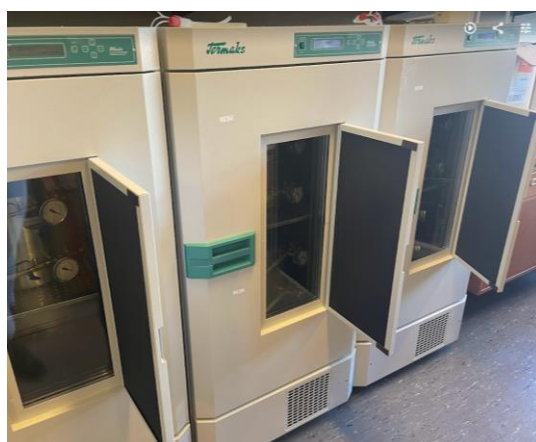
Figure 2.4 Emission sampling system used for identification of VOC emissions from different wood materials.
