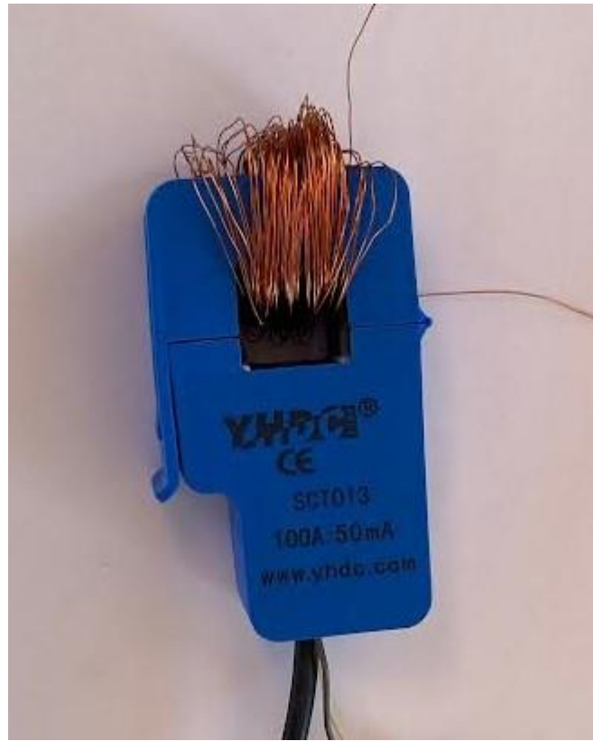
Figure 5 Many turns of enamelled copper wire were wrapped around 50-amp sensors to give a measurable current reading.
