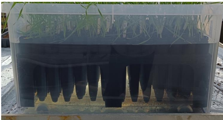
Figure 6. A) White plastic box; B) Waterlogging treatment design complete set-up
