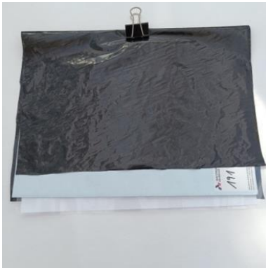
Figure 41. Germination growth pouch with layers of polythene cover, germination paper, and laminated A4 paper stitched with butterfly clip.
