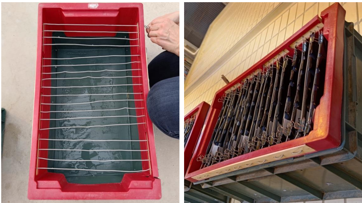
Figure 47: Front view of customized seed growth assembly without growth pouch and side view of it with growth pouch clipped on aluminum wire with butterfly clips. The plastic frame (red color) is placed on top of the plastic tray.
