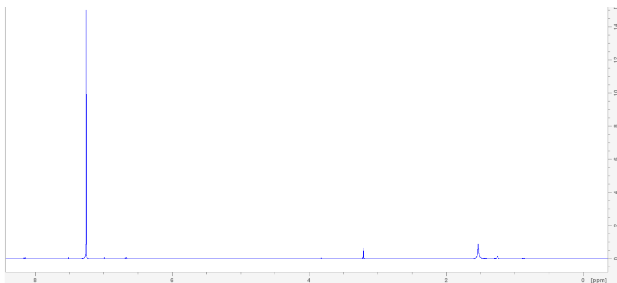
Figure 8: 1 H NMR spectra of the result from the synthesis of (2 E , 4 E )-5-(tert-butyldimethylsilyl) oxy) penta-2,4-dien-1-ol ( 3 ).
