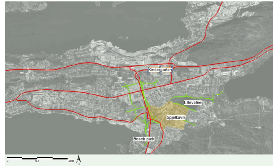
Figure 20: Road Network, Red are the main roads, green are walkways meant for pedestrian and bicycles that are not connected to the main road system.
