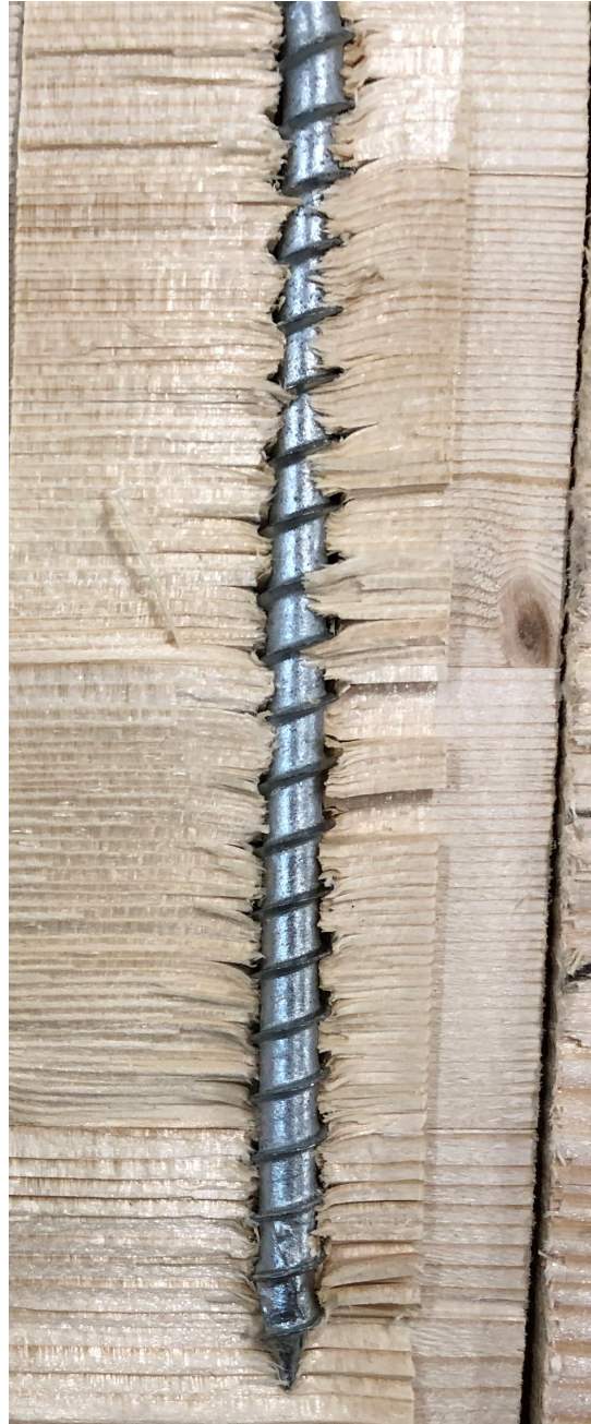
Figure 5.3: Push trough failure
