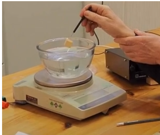
Figure 4.8: Volume measuring using water immersion (10)
