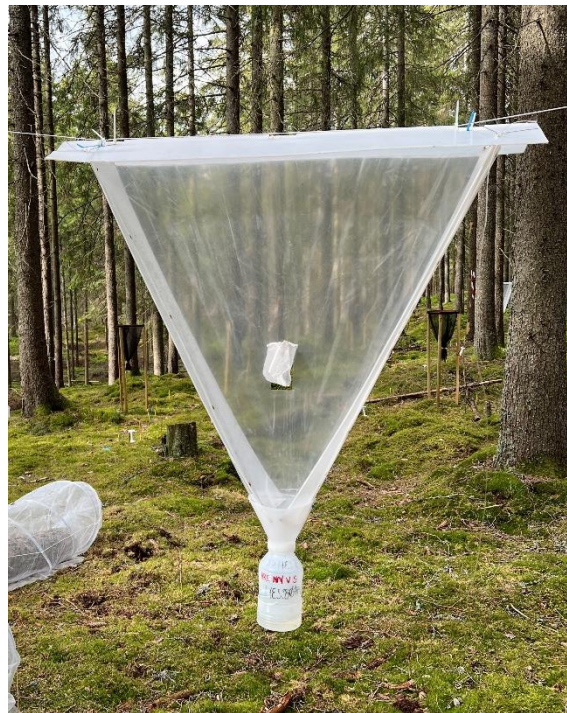
Figure 4. An IBL-2 window trap produced by CHEMIPAN (Warsaw, Poland).
