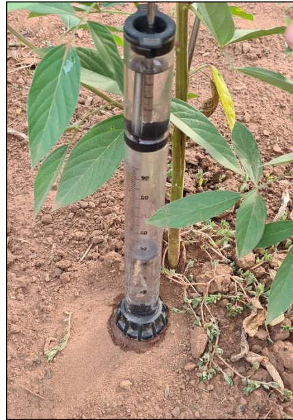
Image 2: Mini Disk Infiltrometer in use at -4 cm pressure. Photo by Adrian Røed Østby.
