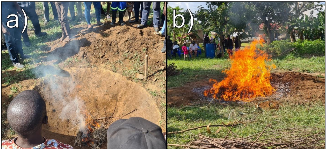
Image 1: a) Start of pyrolysis process in a Kon-Tiki flame curtain kiln in Uganda. b) Flames in the pit consume most oxygen before it reaches a lower level of the kiln. Photos by Adrian Røed Østby.
